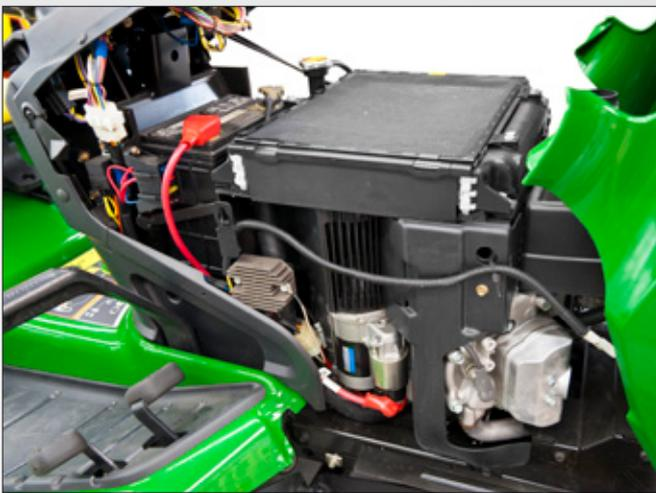
2 cylinder petrol engine, water-cooled 22 HP
